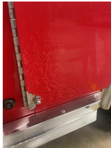
Body Compartment Corrosion
